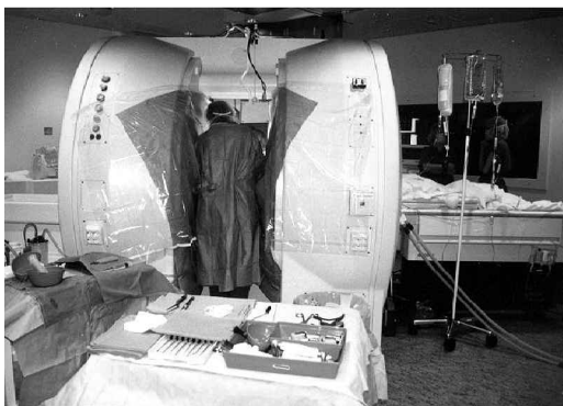
Figure 1. Surgery in the MRI scanner (Signa SP, General Electric). Field strength: 0.5T, vertical gap: 60 cm.
