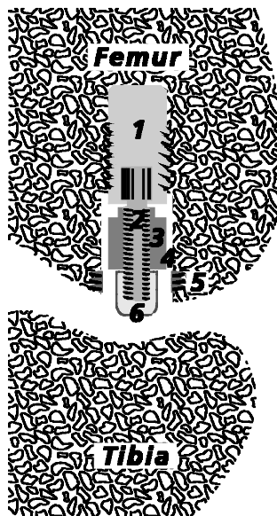
Figure 2. Implant device and test implant positioned in the weight-bearing part of the femoral condyle. 1. Threaded anchorage screw fixed in bone. 2. Threaded piston, which is centered in the drilled hole by the anchorage screw. 3. Test implant mounted onto the piston. 4. Gap measuring 0.75 mm between implant surface and trabecular bone. 5. Titanium ring inserted into the subchondral part of the condyle to prevent early tissue ingrowth to the polyethylene plug. 6. Protrusion of the polyethylene plug (diameter 4.5 mm) which transmits the load from the tibial part of the knee to the implant system. Note the access of joint fluid to the peri-implant gap. Modified after Søballe et al. (1991), Søballe (1993).
