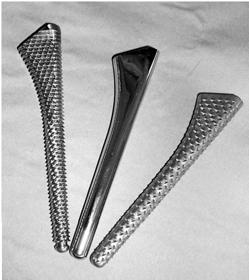
Figure 1. Three different broach configurations used in this study: diamond tooth (left), polished tamp (middle) and chipped tooth (right).
