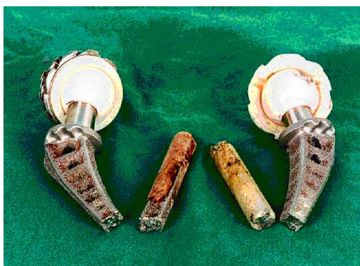
Figure 3. The marble-like appearance of the bone firmly attached to the distal part of both broken stems.
