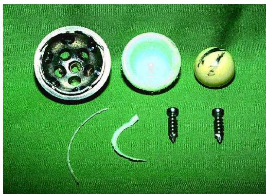
Figure 2. The acetabular cup with metallosis of the ceramic head has been removed. The liner is intact, but the edge is cut off.
