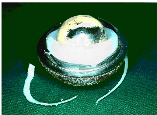
Figure 2. The acetabular cup with metallosis of the ceramic head has been removed. The liner is intact, but the edge is cut off.
