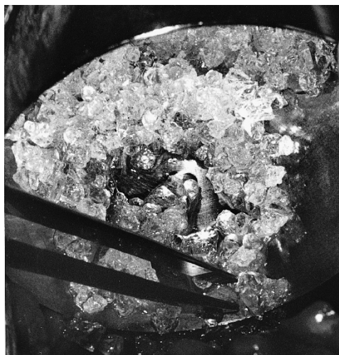
Figure 2. Particulate bioactive glass granules in a container moistened with distilled water.
