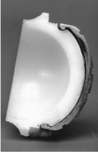
Figure 5. Cross-section of the Howse II metal-backed cup, showing a definite gap between the polyethylene liner and the metal backing.
