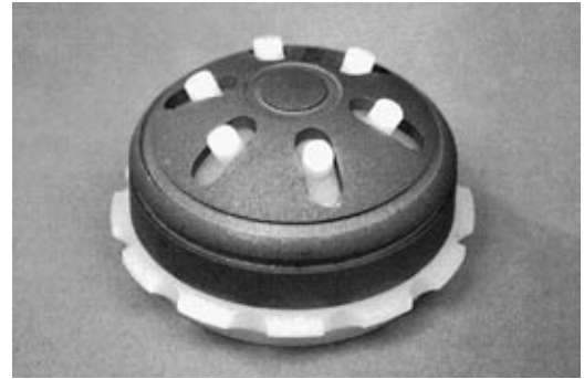
Figure 1. Howse II metal-backed acetabular component showing the characteristics of the cup: titanium metal backing with textured outer surface, small projections of the polyethylene liner acting as cement spacers.
