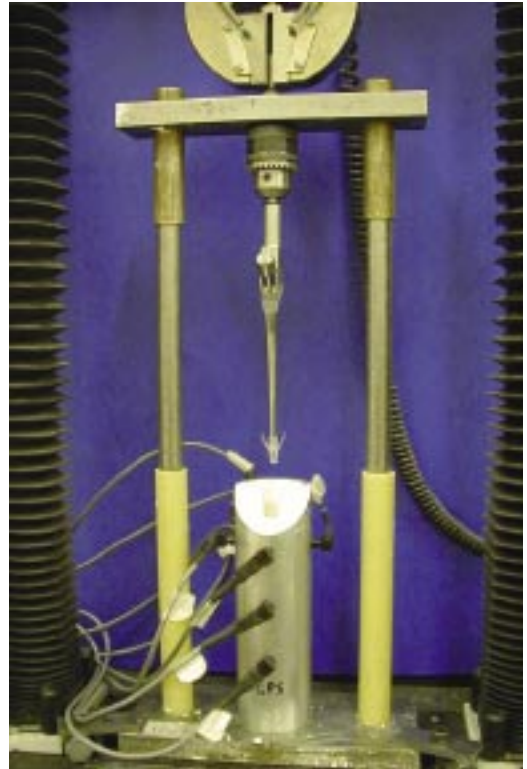
Figure 2. The insertion rig, with prosthesis and model femur in-situ, positioned in the Instron materials testing machine.
