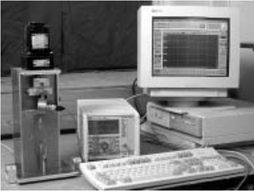
Figure 10. The "home-made" materials testing machine used in the first 3 studies.
