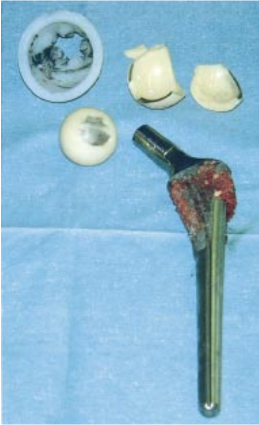
Figure 4. Retrieved implant showing fractured insert, but intact femoral head.
