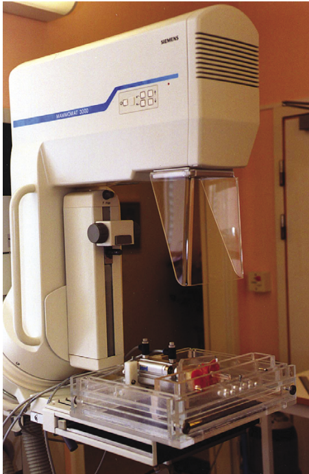
Figure 1. The experimental set-up. Exposure on the high resolution mammography x-ray film with the bone pieces under continuously pressure of the pneumatic piston with 40 kPa.
