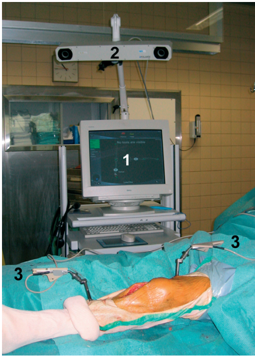
The navigation system. 1 = monitor, 2 = infrared camera, 3 = light-emitting diods.
