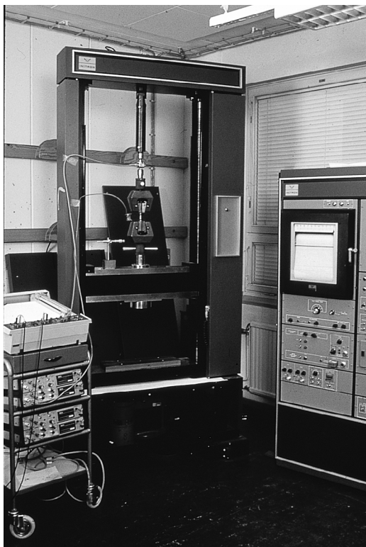
Figure 8. Instron testing-machine with a cement bar mounted as in study II.
