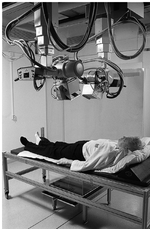
Figure 11. Patient in position for RSA examination with the two X-ray tubes above and the calibration cage beneath the patient.
