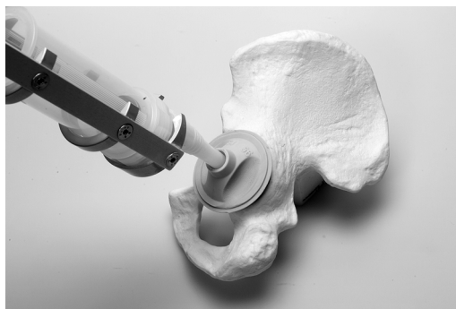
Figure 3. Illustration of the compressor used for the second phase of a sequential cementation in studies IV and V.
