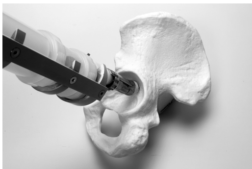
Figure 2. Illustration of the injector used for initial cementation of the anchorage holes during sequential cementation in studies IV and V.
