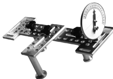
Figure 4. Construction of the inclinometer. There are 3 ultrasound markers and an angle measurer fixed to the instrument.
