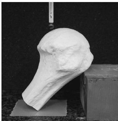
Figure 1. The device used for three-dimensional morphological analysis. This is only a sample picture. This humerus is not a real one for measurement, but a dummy bone. All specimens were fixed so that the articular surfaces faced upwards, and they were measured at intervals of 0.3 mm on the articular surfaces and 1 mm at the shafts.
