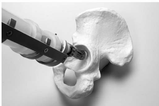
Figure 1. a. The injector used for initial cementation of the anchorage holes during sequential cementation.
