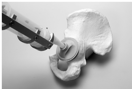
b. The compressor used for the second phase during sequential cementation
