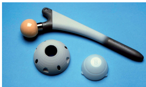
Figure 1. The uncemented total hip replacement device with a straight, collarless stem made of a titanium-aluminium-vanadium alloy (Ti-6Al-4Va), with an additional coating of hydroxyapatite in the proximal two-thirds, which was combined with spherical press-fit cup (Ti-6Al-4Va), a polyethylene liner and a ceramic head.
