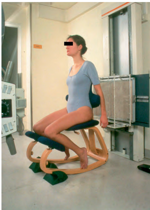
Figure 1:4C. RSA in sitting position on a chair with standardized lowering of the knees allowing free passage of the x-rays above the femoral shafts to the lumbosacral spine. (Reproduced with permission from Spine).
