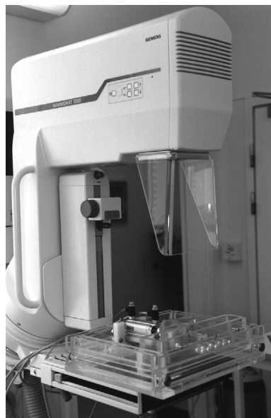
Figure 3. Experimental setup. Radiographic examination of specimen during a continuous force of 330 N.
