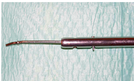
Figure 3. The photograph demonstrates how a ball-tipped guide wire is passed through the nail. A 3.5-mm screw is placed in one of the distal holes which will lock the guide wire during extraction.
