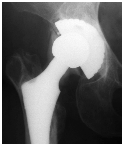
Figure 1. Anteroposterior radiograph taken 25 months after revision because of ceramic liner fracture, demonstrating metallosis around the stem neck. Note the loss of the superior part of the cobalt-chromium head.
