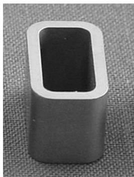
Figure 1. The titanium cage used for all experiments in this study. The external dimensions are 10 \times 10 \times 18 mm. The wall thickness is 1.5 mm. The same cage, made of both titanium and several bioresorbable polymers, has been used in earlier in vivo studies in the goat.
