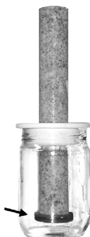
Figure 2. Fat separator consisting of a perpendicular Plexiglas cylinder filled with morsellized bone. Fat is drained by gravity through a stainless steel mesh at the bottom (arrow). To facilitate fat drainage by reducing viscosity, the separator was kept in an incubator (40°C).
