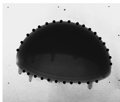
Figure 5. Trilogy cup dots marking the contour of the cup (hemispherical cup algorithm).
