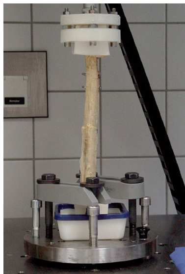
Figure 5. Torsional testing with a torsional moment of 6.5 Nm.
