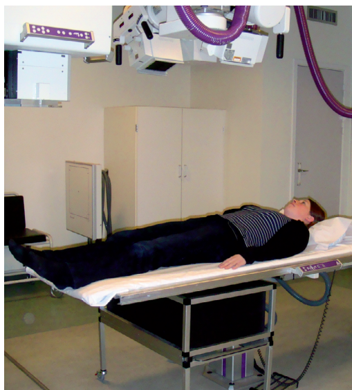
Figure 19. The RSA set-up with the patient positioned supine on the examining table and a calibration box underneath creating a 3D coordinate system of tantalum markers.
