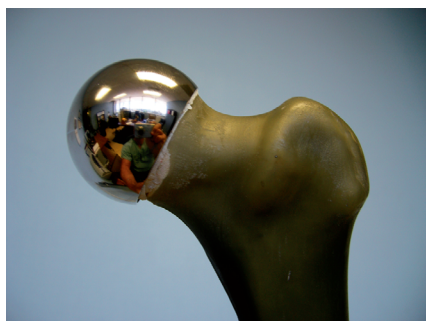
Figure 1. A synthetic composite model femur with a femoral resurfacing component implanted to optimize fixation and minimize bone loss.
