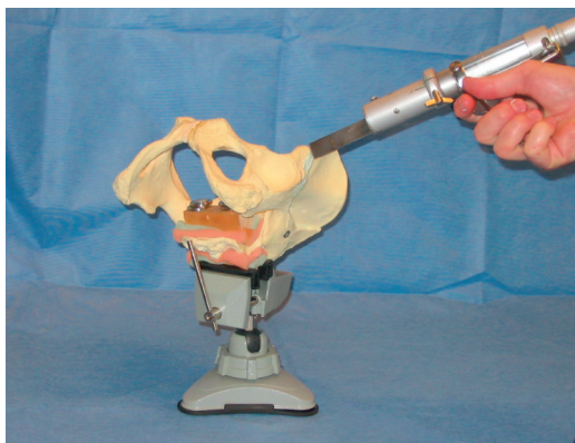
Figure 2. The sawbone is rigidly fixed by a steel clamp with a 360° rotational base. The cutting is performed using an oscillating saw.
