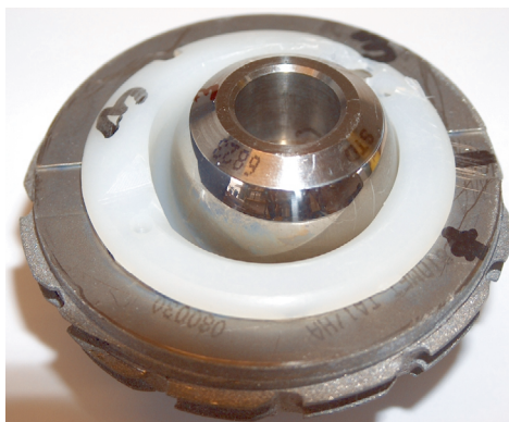
Figure 1. Acetabular cup, polyethylene liner, a titanium shell (52–58 mm outer diameter), and a femoral head (28 mm).
