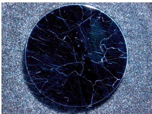
Figure 4. Macrostructure of a cross section taken through the neck of a fractured stem. Note the large grains and the presence of precipitates at the grain boundaries.
