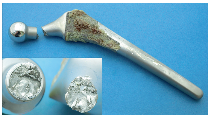
Figure 1. Macro photograph of fractured stem. Insert shows surface of fracture.
