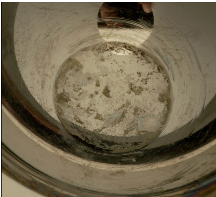
Figure 2. Explanted McKee-Farrar acetabular component (size 41.5 mm). All explanted prostheses showed layers that were visible to the naked eye. The morphology of the layers was inhomogeneous. Samples were cut into several smaller pieces for further evaluation.
