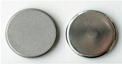
Figure 1. Titanium discs (left) and steel alloy discs (both from Scandinavian Customized Prosthesis AS, Trondheim, Norway) served as surfaces for biofilm formation, with roughness of R_a = 2.5 \mu\text{m} and R_a < 0.5 \mu\text{m} for titanium and steel discs, respectively. All discs were manufactured with a diameter of 17 mm and a thickness of 2 mm.
