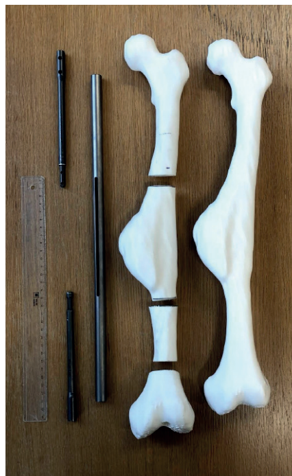
Figure 2. 3-D printed model for testing the setup.
