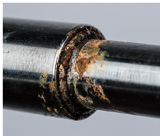
Figure 3. Discoloration at the telescoping interface of a removed Stryde nail.
