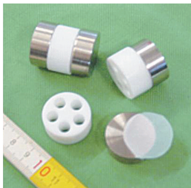
Figure 5. Moulds according to ISO 5833 to produce cylindrical 6x12 mm test specimens.
