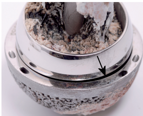
Figure 4. Macroscopic wear (arrow).
