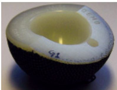
Figure 1. Polyethylene acetabular cup with titanium mesh molded on the outside.
