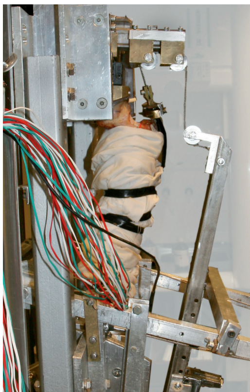
Figure 6. Photo illustration of a femur mounted in the hip simulator.
