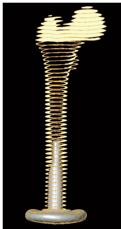
Figure 12. Preoperative computer-based construction of the femoral endoprosthesis inside the residual femur.
