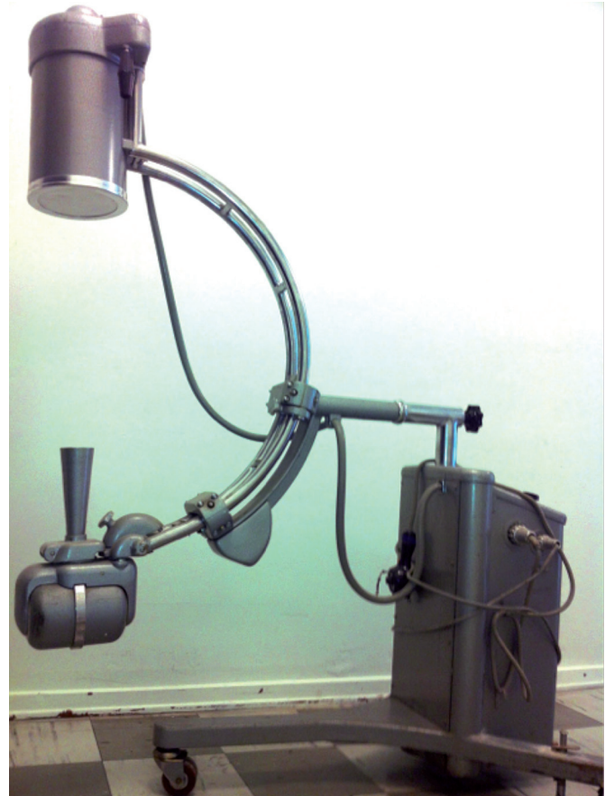
Figure 2. The introduction of the C-arm image intensifier in the 1950s and -60s made the use of closed x-ray guided nailing safer for the surgical staff. Before this you would wear a box on your head with a piece of fluorescent glass in front of your eyes. The x-ray beam would be aimed straight at your face. The picture shows the Philips BV20 C-arm introduced in 1955 and in use until the late 1960s. This one was used at Haukeland University Hospital. (Photo Sven Young)
