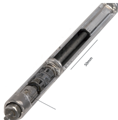
Figure 1. A PRECICE nail transected with a laser. The integrated magnet (arrow) is visible on the threaded rod.
