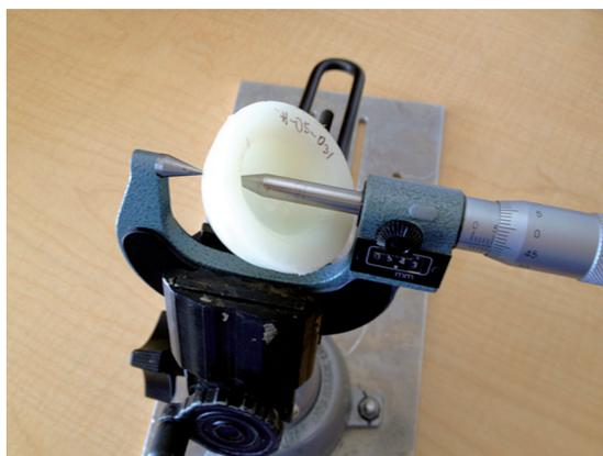
Figure 3. The cup wall thickness measurement setup showing the point micrometer, cup, and holding apparatus.
