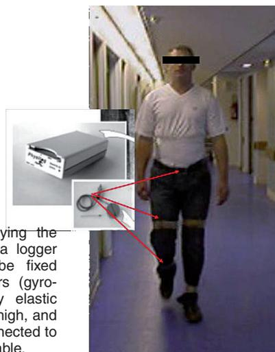
Figure 1. A subject carrying the Physilog system. The data logger (weighing 300 g) can be fixed around the waist. Sensors (gyroscopes) are attached by elastic strips to each shank and thigh, and also to the pelvis, and connected to the data logger by a thin cable.
